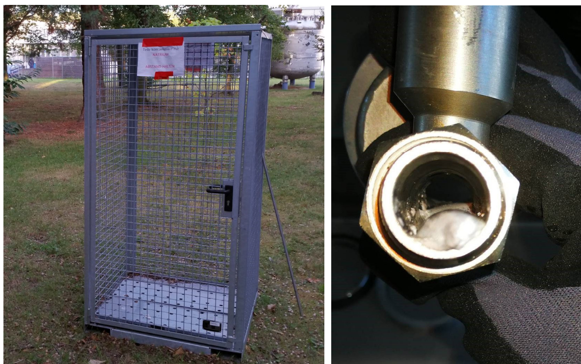
Figure 4.1 Lattice box for cleaning of small components (left) and partially blocked pipe (right)
