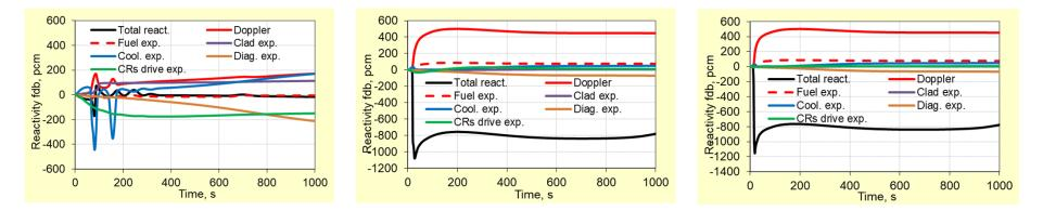
Conclusion: Both options are capable to shutdown ESFR in a timely manner, in order to avoid the negative consequences of the base ULOOP transient.
