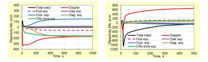
Conclusion: DSD rods (CPEM option in this case) are capable to shutdown ESFR in a timely manner, in order to avoid the negative consequences of the base UTOP transient.
