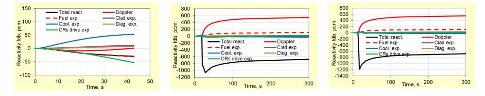
Conclusion: Both PSS options are capable to shutdown ESFR in a timely manner, in order to avoid the negative consequences of the base ULOF transient.
