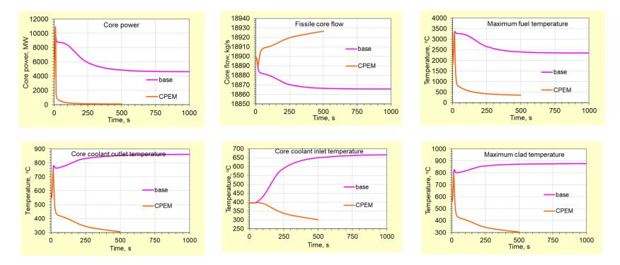
of positive reactivity insertion, activation of the DSD rods shutdown the reactor and all core and primary cooling circuit temperatures decrease. No local fuel melting takes place in the reactor core.
