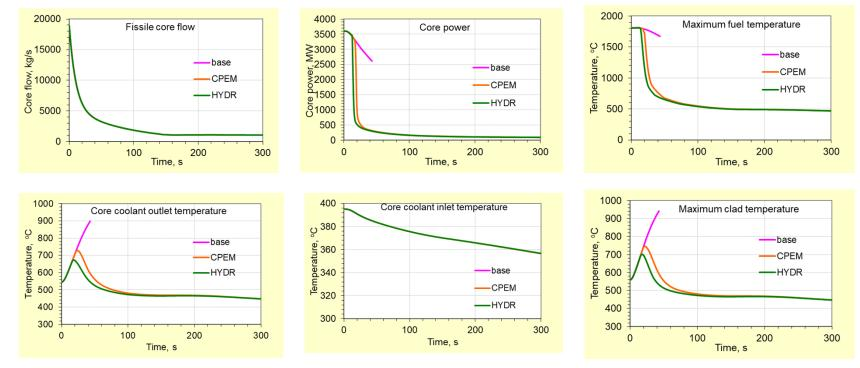
Base case: Sodium at the outlet of the core for the peak power channel starts boiling at  $t\sim43$  s into the transient. Peak-power pin clad failure is predicted at  $t\sim60$  s into the transient.
