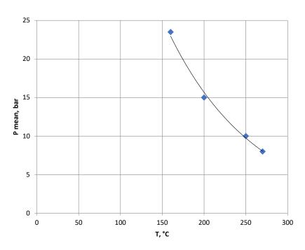
Pressure oscillation amplitude as a function of TAc mean pressure
