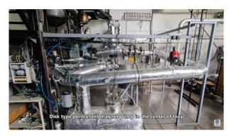
A new liquid sodium loop with intelligent pump control system built in IPUL during 2020
