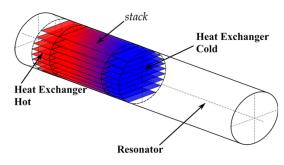
Thermoacoustic effect in a pipe with limited distance – induction of sound wave
