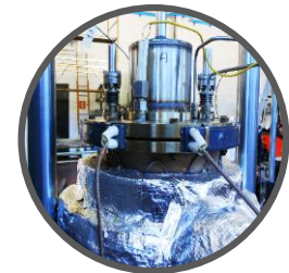
Fretting tests in lead alloy
